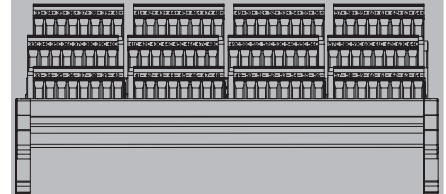
Field terminals view for ADV161 (Channels 33 to 64)
